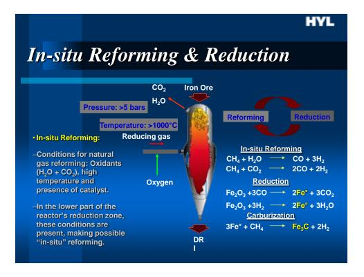
Reforming of natural gas requires: A certain level of oxidants ( $H_2O$  and  $CO_2$ ), which have to be carefully controlled; a high temperature, as a result of partial combustion; and an active catalyst, which is provided by the metallic iron units from the iron ore already reduced.
