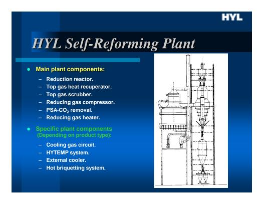
In the HYL self-reforming plant, the main components are the following: Reduction reactor, top gas heat recuperator, top gas quenching/scrubbing system, reducing gas recycle compressor,  $CO_2$  removal system and reducing gas heater.
