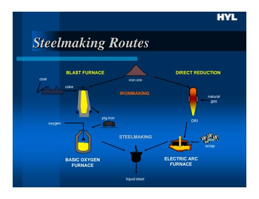
There exist in the world two main routes for the production of liquid steel: On one side, the "Classical Route" based on blast furnace ironmaking and conversion of pig iron to steel. On the other side, the "Modern Route" for the production of steel in electric arc furnaces, using as raw material either scrap or Direct Reduced Iron (DRI).
