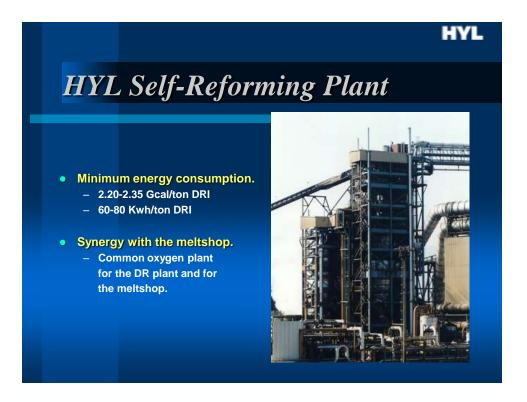
The overall energy efficiency of the self-reforming process is optimized, by the integration of partial combustion, pre-reforming and catalytic reforming inside the reactor, as well as by a minimum utilization of thermal equipment in the plant. Therefore, most of the energy supplied to the process is taken by the product, with minimum energy losses to the environment.
