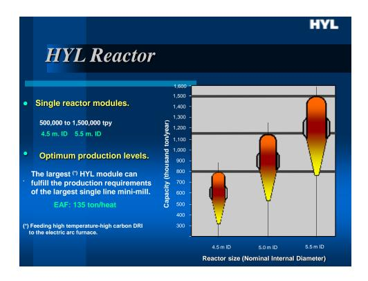
Based on single reduction units, HYL plants are designed for capacities ranging between 300,000 and 1,500,000 ton/year of DRI/HBI. There are three standard HYL reactor sizes (4.5 m ID, 5.0 m ID, and 5.5 m ID), which can be specified according to the required production capacity for each project.
