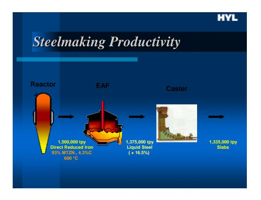
However, when 100% high carbon-high temperature DRI is fed, with 93% metallization, 4.3% carbon and 600 °C, the furnace productivity is dramatically increased, reaching a liquid steel production of 1,375,000 ton/year in the reference EAF. Compared to the operating practice using 70% scrap and 30% DRI/HBI, the productivity is increased by 17%. In this case, the slab production is about 1,335,000 ton/year.
