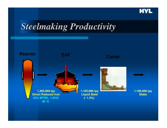
In case of a mini-mill feeding 100% cold DRI to the EAF, with 93% metallization and 1.8% carbon, the maximum liquid steel production for the reference EAF is about 1,165,000 ton/year of liquid steel. This means that the productivity of the EAF is very similar (1.3% lower) to that obtained in an operating practice feeding 70% scrap and 30% DRI/HBI. In this case, the slab production is about 1,100,000 ton/year.
