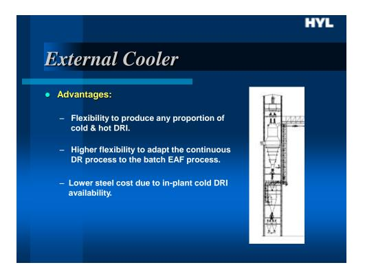
Hot DRI is discharged by means of the reactor rotary valve, through the diverter valve, which delivers material either to the HYTEMP system or to an alternative external cooler (for cold DRI production). The pneumatic transport is normally carried out at the same rate as the reactor production rate.
