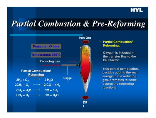
In general, partial combustion of natural gas with oxygen provides the additional energy, which is required for natural gas reforming in-situ, and for the carburization of the metallic iron, eliminating the need of a natural gas-steam reformer.
