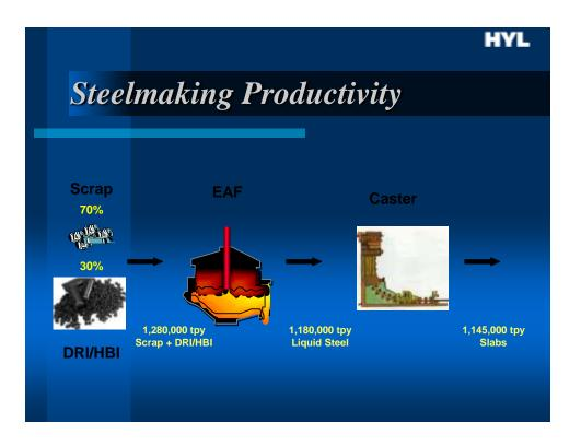
In a typical flat product mini-mill, using 70% scrap and 30% DRI/HBI, the maximum liquid steel production which can be attained in the reference EAF (135 ton of liquid steel per heat) is about 1,180,000 ton/year of liquid steel. The corresponding slab production is about 1,145,000 ton/year.
