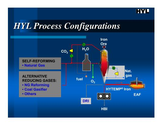
One of the main advantages of the HYL process is its configuration based on independent reducing gas generation and reduction sections. Under these conditions, the only requirement is an independent source to supply the  $H_2$  and CO needed for reduction, with no changes involved in the process scheme.
