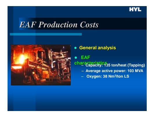
In order to evaluate the benefits of the use of high temperature-high carbon DRI on the production of liquid steel, an state of the art-EAF has been considered for all cases with the following characteristics:
