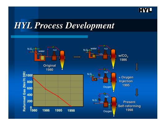
The first industrial plant operating with the HYL moving bed process started up in May, 1980, based on a process concept oriented to high plant productivity and superior DRI quality, low energy consumption, and a simpler operation. Through the years, several improvements have been incorporated in the moving bed process, thus optimizing the process efficiency and plant reliability.
