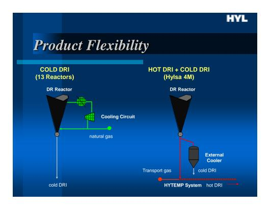
The flexibility of the HYL direct reduction process, for the production of different product types and combinations of them, can be illustrated by the following examples of HYL plants in operation:
