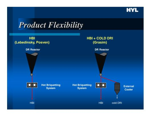
Hot Briquetted Iron (HBI). HBI is produced from hot discharged DRI (700 °C), and is more commonly used for overseas export. HBI can also be produced when low quality friable iron ores are to be processed, and these ores cannot be used for the production of cold DRI.
