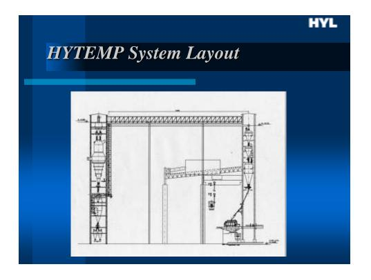
The HYTEMP system involves an HYL hot discharge direct reduction reactor, connected to an adjacent electric arc furnace mill by means of a pneumatic transport system.
