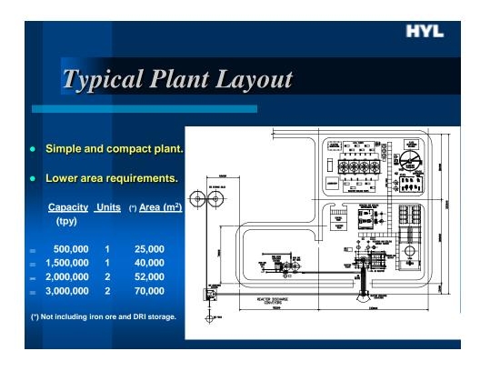
HYL plants are simple in design and compact facilities, as can be observed in the typical layout for a plant design based on the self-reforming scheme.
