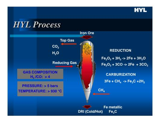
The HYL process was designed for the direct reduction of iron ores, using reducing agents such as hydrogen  $(H_2)$  and carbon monoxide (CO).
